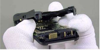
Before loosening the upper snaps of the cover be sure that you press the module against the A-Cover. The module is still fixed with the A-Cover with one hidden screw in the antenna area.
