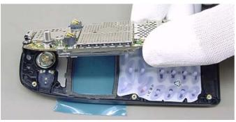
Lifting up the CMT module is very easy now. Protect the display with a foil.
