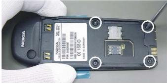
To open the unit, four T6 screws have to be opened. Do not use your torque driver for this, because torque drivers are mostly designed for fastening and not for opening screws.
