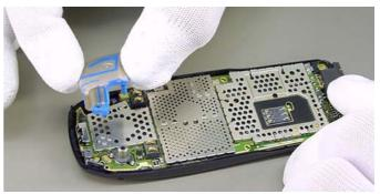
Don't touch the Antenna with your fingers. The fingerprints would cause corrosion to this sensitive material.
