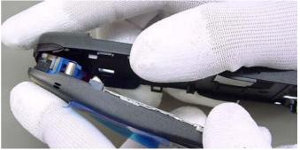
Now you can take away the B-Cover. Be careful not to damage the antenna, which can break if you try to rotate the cover against each other.
