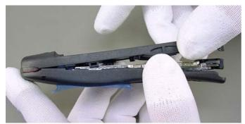
Hold the unit with the Volume Key against the table. Hold the A-Cover with your left hand and then grab the B-Cover to unlock the side snaps in the bottom area.
