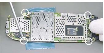
Four clear plastic clips hold the UI module on the CMT module. Unlock these clips when you need to remove the UI module.
