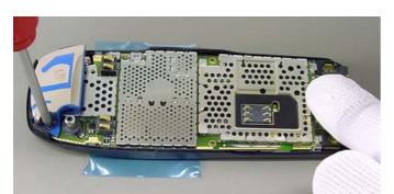
This is the screw, which fixes the Antenna and holds the module inside the A-Cover.
